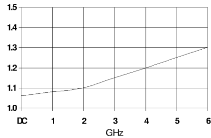
On Port Input/Output VSWR vs. Frequency V Control = -5 V
