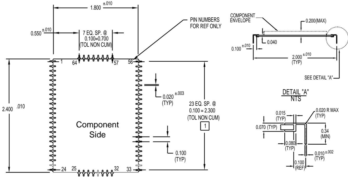
**FIGURE 3A. DD-42900DP DIP MECHANICAL ASSEMBLY**
