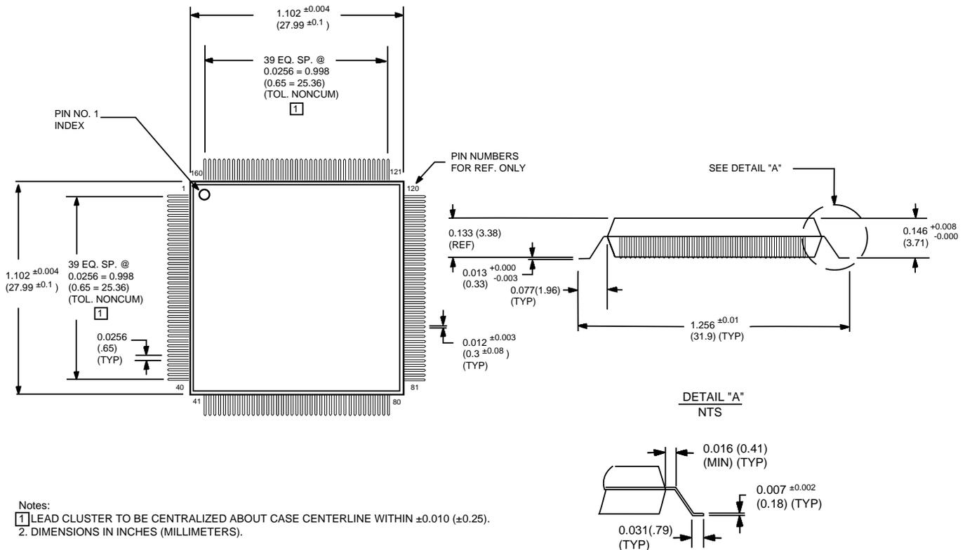
FIGURE 2. DD-00429FP ASIC MECHANICAL OUTLINE (PLASTIC)
