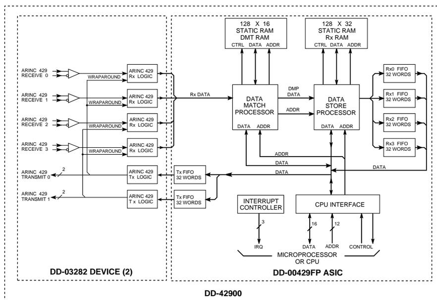
FIGURE 1. DD-42900 BLOCK DIAGRAM
