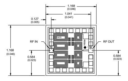
THREE PADS ON EACH CORNER MUST BE BONDED TO GROUND (12 TOTAL).
