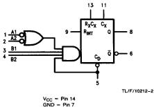
GND = Pin 7 NC = Pins 10 and 12
