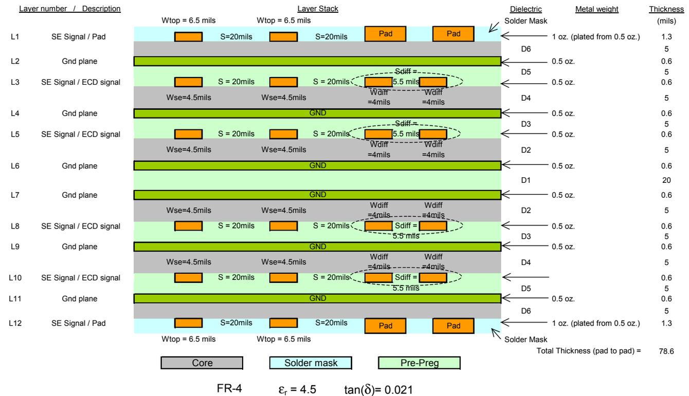
Figure 6. Warplink Test Card Layer Stackup
