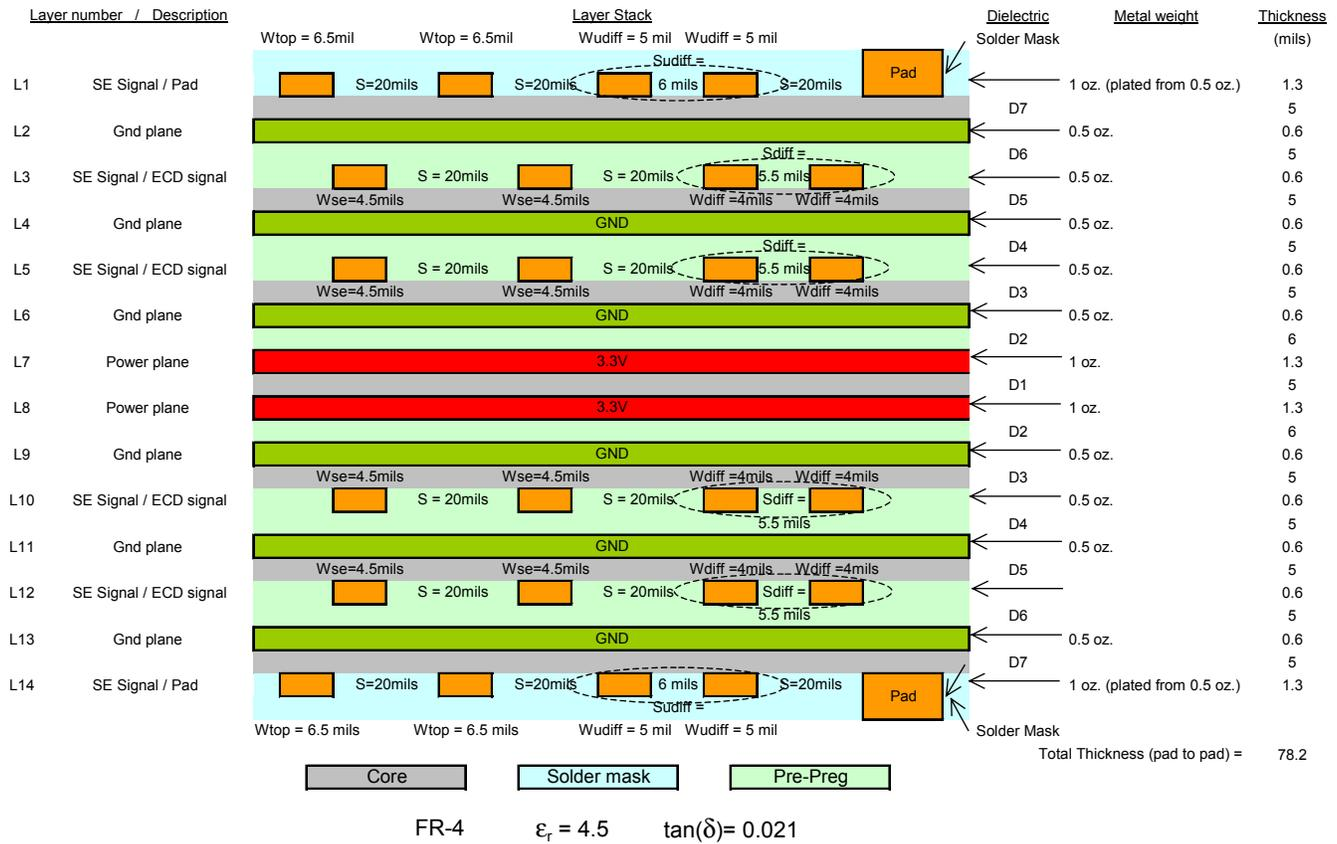
Figure 7. Warplink Line Card Layer Stackup
