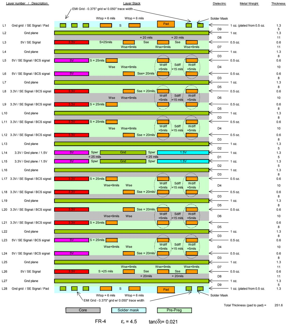
Figure 5. WarpLink Reference Backplane Layer Stackup
