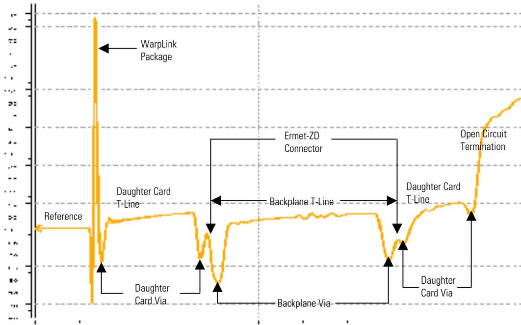
Figure 12. TDR of 10-inch Backplane with Through Vias
