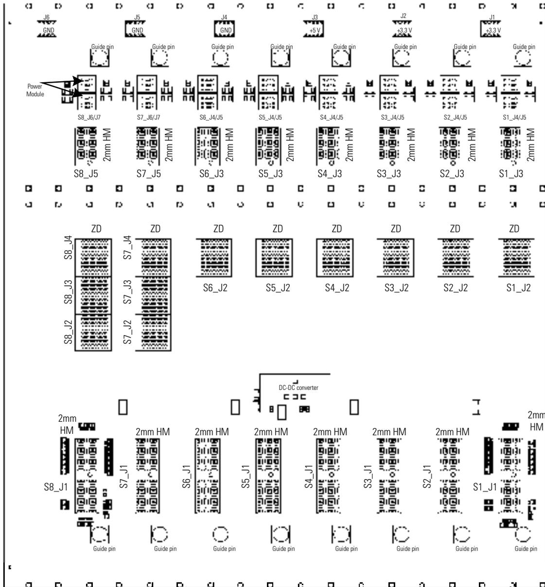
Figure 4. WarpLink Reference Backplane (Front View)
