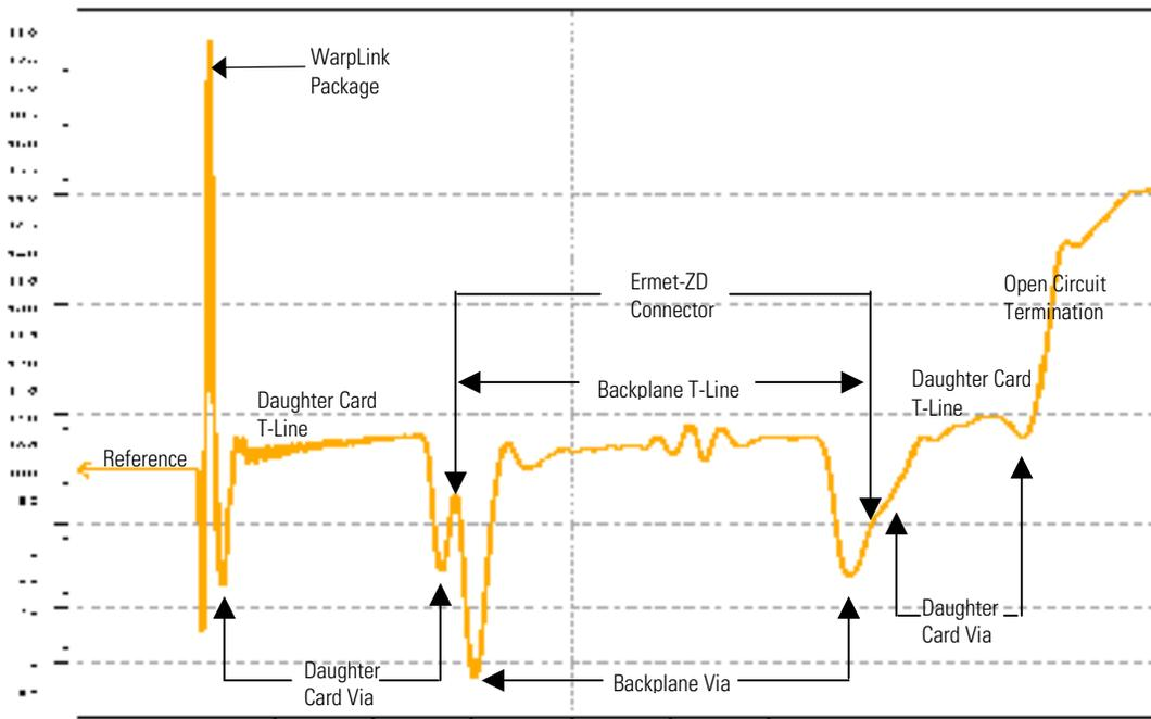
**Figure 11. TDR of 10-inch Backplane with Via Stubs**
