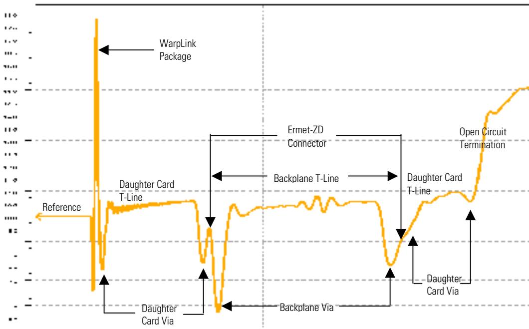
Figure 14. Simulated TDR of 10-Inch Backplane with Via Stubs
