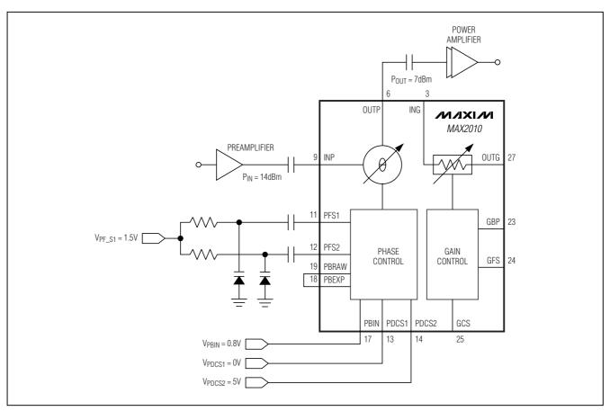
Figure 4. AM-PM Response Tuning Circuit
