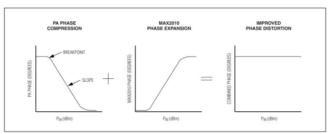
Figure 1. PA Phase Compression Canceled by MAX2010 Phase Expansion
