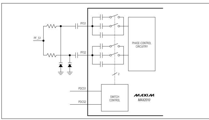
Figure 2. Simplified Phase Slope Internal Circuitry
