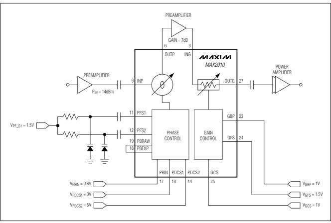
Figure 5. MAX2010 Phase and Gain Optimization Circuit
