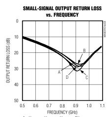
A = V<sub>PDCS1</sub> = V<sub>PDCS2</sub> = V<sub>PF\_S1</sub> = 0V B = V<sub>PDCS1</sub> = V<sub>PDCS2</sub> = 0V, V<sub>PF\_S1</sub> = 5V C = V<sub>PDCS1</sub> = V<sub>PDCS2</sub> = 5V, V<sub>PF\_S1</sub> = 0V D = V<sub>PDCS1</sub> = V<sub>PDCS2</sub> = V<sub>PF\_S1</sub> = 5V
