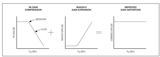
Figure 3. PA Gain Compression Canceled by MAX2010 Gain Expansion
