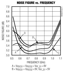
$C = V_{PDCS1} = V_{PDCS2} = 5V$ ,  $V_{PF\_S1} = 0V$  $D = V_{PDCS1} = V_{PDCS2} = V_{PF\_S1} = 5V$
