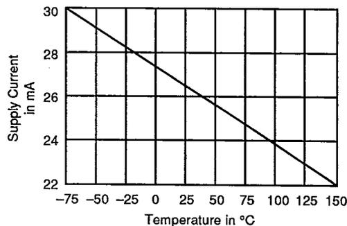
**Figure 2. Typical Supply Current vs. Temperature**
