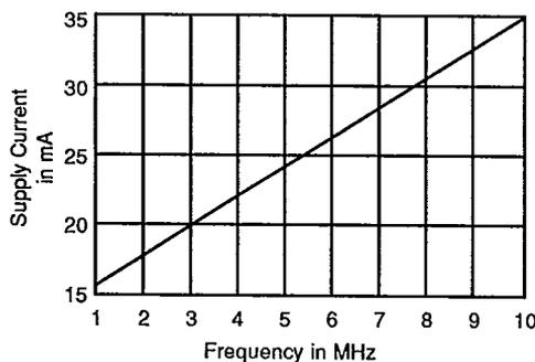
**Figure 1. Typical Supply Current vs. Frequency**
