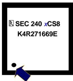
For consumer package, pin #1 (ROW 1, COL A) is located at the A1 position on the top side and the A1 position is marked by the marker “●”.
