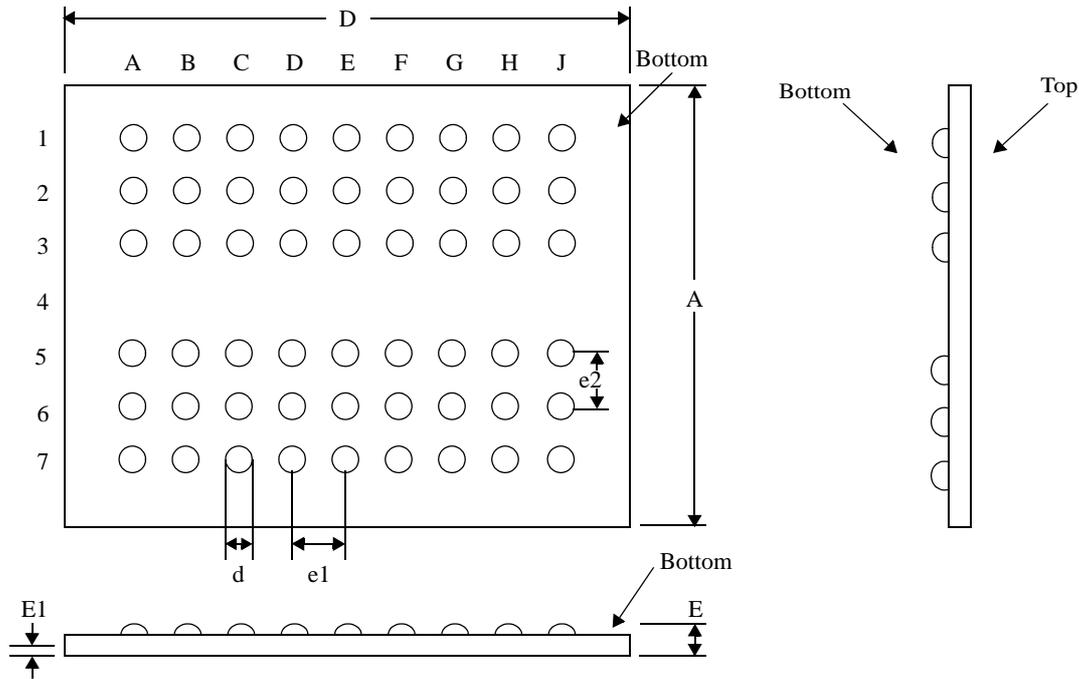
**Figure 4: Center-Bonded Fanout CSP Package**
