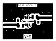
Optimised PCB layout for SAW filters in QCC8C package, pinning 1,5 (top side, scale 1:1)
