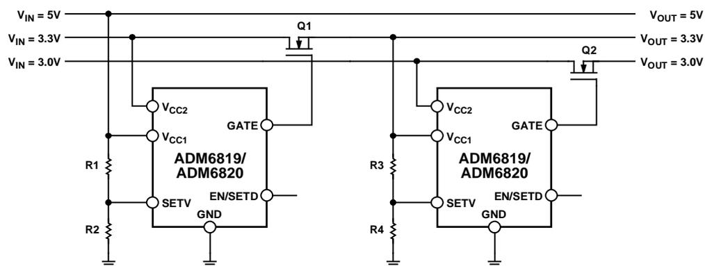
Figure 5. ADM6819/ADM6820 Solution for Sequencing Three Supply Rails
