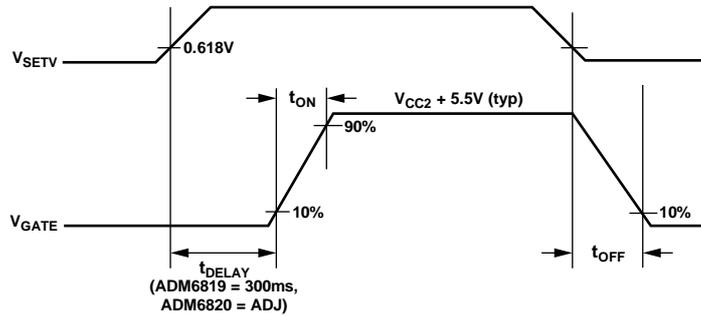
Figure 3. ADM6819/ADM6820 Timing Diagram Using SETV for Sequencing
