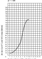
Adjustable Restrictor Valves 1/4 (DN3.5) Supply pressure = 7 bar  $\Delta p = 1$  bar
