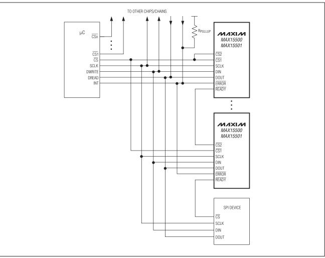
Figure 6. Daisy-Chain Terminating (Compatible with Standard SPI)
