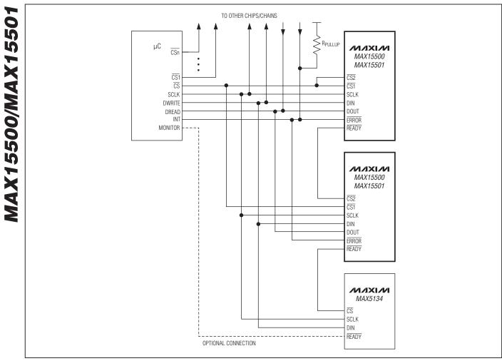
Figure 7. Mixed MAX15500/MAX15501 and MAX5134 Daisy-Chain Connections
