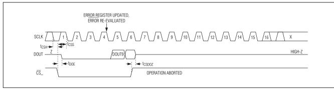
Figure 10. Aborted SPI Programming Operation (Invalid, Showing tCSDOZ and Internal Activity)
