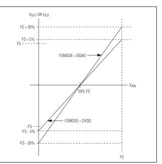
Figure 2. Bipolar Transfer Function
