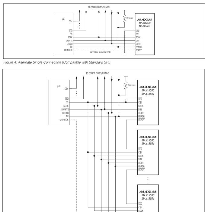
Figure 5. Daisy-Chain Connection (Compatible with Standard SPI)
