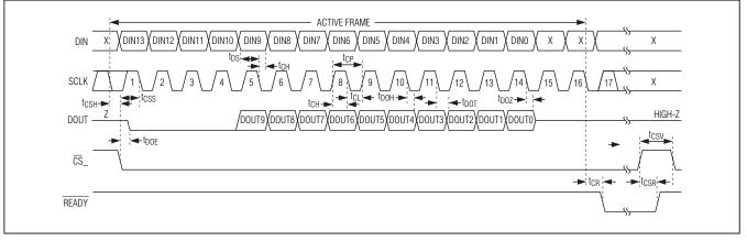
Figure 9. Extended SPI Programming Operation (Daisy-Chained Applications)
