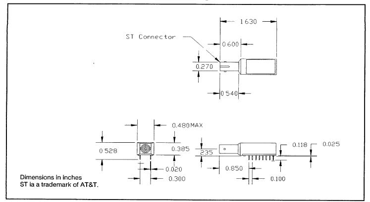
The package provides molded-in standoffs to allow for proper cleaning beneath the part after soldering. Parts are shipped with a protective cap
