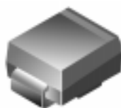
SMB/DO-214AA COLOR BAND DENOTES CATHODE
