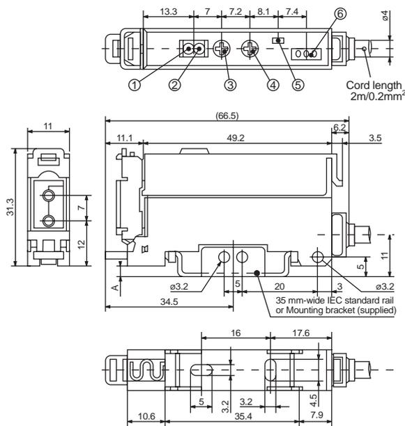
maximum mounting screw torque 1Nm
