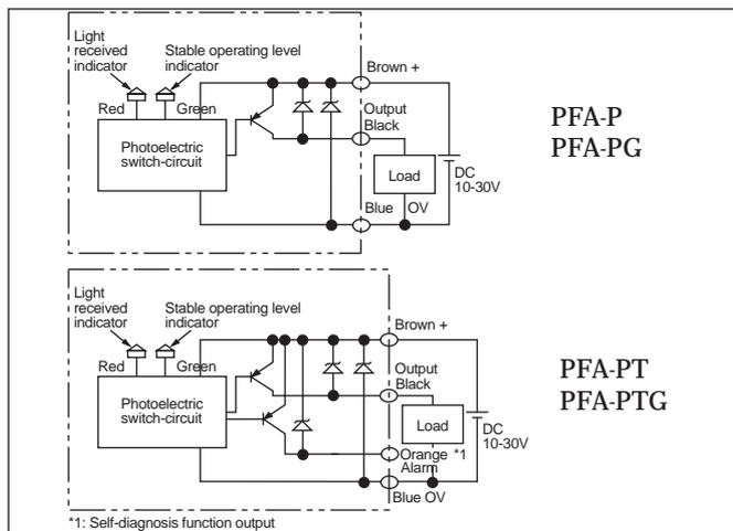
Note: the +V, output and OV (gnd) connections are also available on the top of the amplifier in the form of terminals, for operation check (test) purposes.
