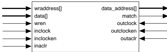
Figure 23. APEX 20KE CAM Block Diagram
