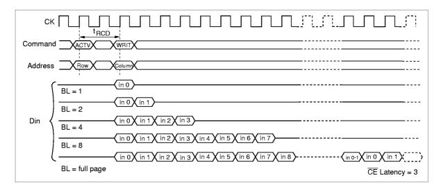
**2. Single write:** A single write operation is enabled by setting OPCODE (A9, A8) to (1, 0). In a single write operation, data is only written to the column address and the bank select address (BA) specified by the write command set cycle without regard to the burst length setting. (The latency of data input is 0 clock).
