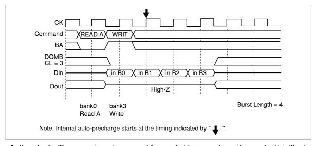
**2. Same bank:** The consecutive write command from read with auto precharge (the same bank) is illegal. It is necessary to separate the two commands with a bank active command.
