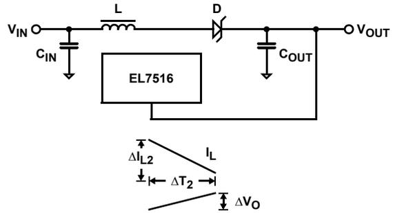
FIGURE 31. BOOST CONVERTER - CYCLE 2, POWER SWITCH OPEN
