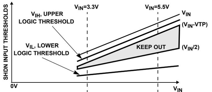
FIGURE 32. SHDN INPUT THRESHOLD vs INPUT SUPPLY VOLTAGE
