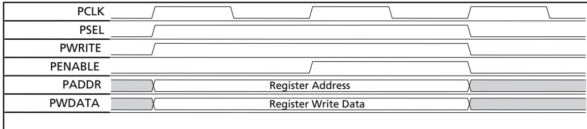
Figure 1-8 · Data Write Cycle
