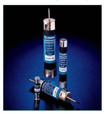
KLNR/KLSR series RK1 fuses were the earliest type of current-limiting fuses developed. Their single-element, silver link design enables them to provide fast-acting overload and short-circuit protection. When used to protect inductive loads such as motors, solenoids, and transformers, KLNR/KLSR series fuses must be greatly oversized to prevent opening the fuses on harmless in-rush currents. In such applications, KLNR/KLSR series fuses may only provide short-circuit protection.
