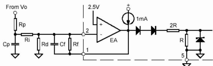
Error Amp compensation circuit for stabilizing current-mode boost and flyback topologies operating with continuous inductor current.
