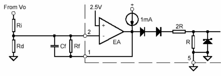
Error Amp compensation circuit for stabilizing any current-mode topology except for boost and flyback converters operating with continuous inductor current
