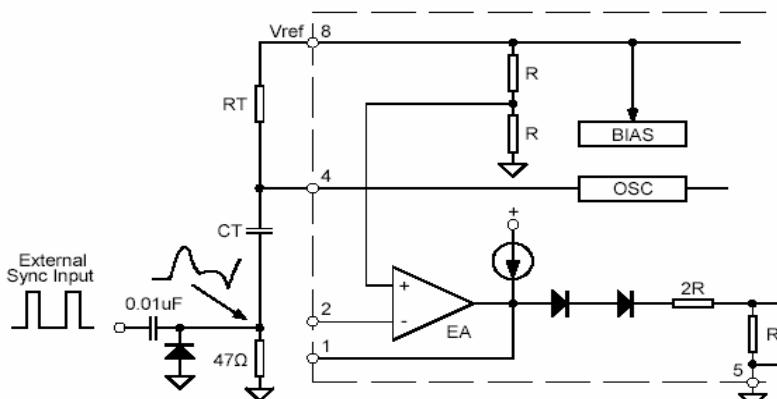
The diode clamp is required if the Sync amplitude is large enough to cause the bottom side of CT to go more than 300mV below ground
