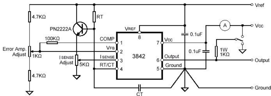
High peak currents associated with capacitive loads necessitate careful grounding techniques. Timing and bypass capacitors should be connected close to pin5 in a single point ground. The transistor and  $5\text{K}\Omega$  potentiometer are used to sample the oscillator waveform and apply an adjustable ramp to pin3.
