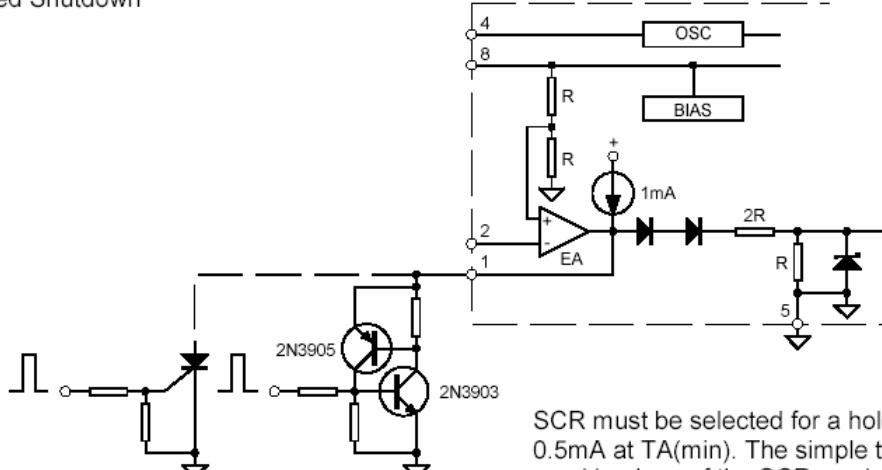
SCR must be selected for a holding current of less than 0.5mA at TA(min). The simple two transistor circuit can be used in place of the SCR as shown. All resistors are 10K.
