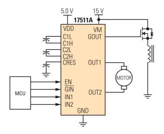
Figure 1. 17511A Simplified Application Diagram
