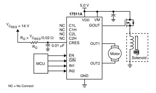
Figure 7. 17511A Typical Application Diagram
