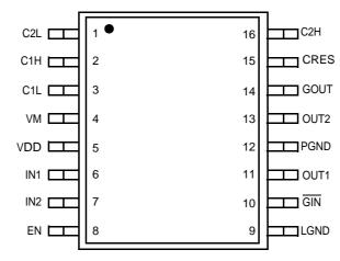
Figure 3. VMFP Pin Connections
