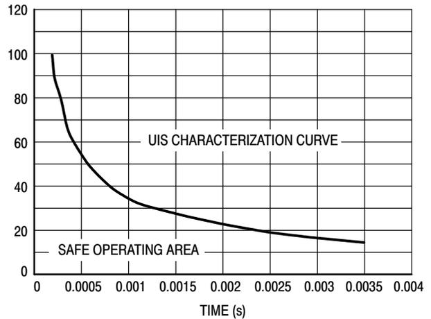
**Figure 12. Peak Reverse Current versus Time for DUT**
