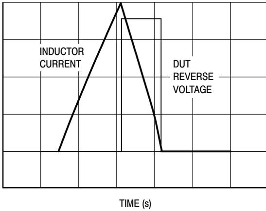
**Figure 11. Typical Voltage and Current UIS Waveforms**
