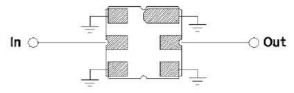
Source/ Load Impedance = 50 ohms
