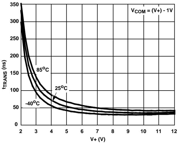
FIGURE 15. ADDRESS TRANS TIME vs SUPPLY VOLTAGE
