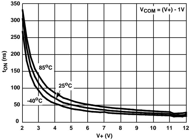
FIGURE 13. TURN - ON TIME vs SUPPLY VOLTAGE
