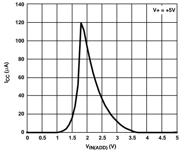
FIGURE 12. SUPPLY CURRENT vs DIGITAL ADDRESS INPUT VOLTAGE
