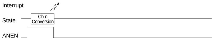
Figure 6-1-3 One Channel/Single Conversion Timing
