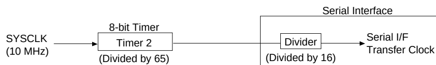
Figure 5-2-1 Asynchronous Transmission Configuration
