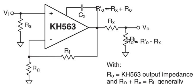
**Figure 9: Improving Output Impedance Match vs. Frequency**
