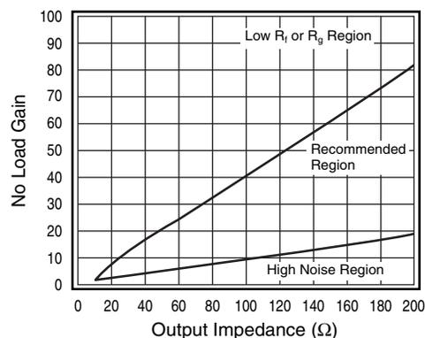
**Figure 7: Recommended Gain and Output Impedance Range**
