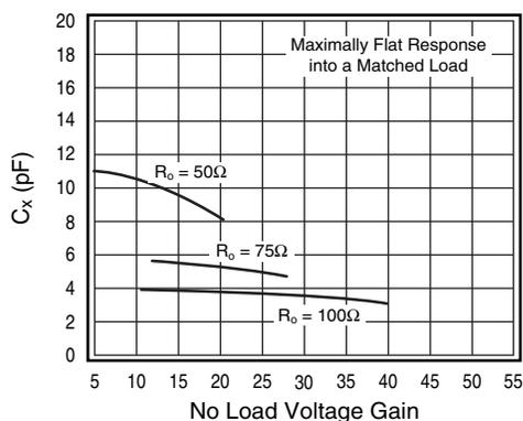
**Figure 6: External Compensation Capacitance ( $C_x$ )**
