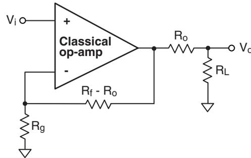
$$\frac{V_o}{V_i} = \left( 1 + \frac{R_f - R_o}{R_g} \right) \frac{R_L}{R_L + R_o}$$
