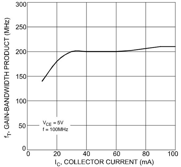
Fig. 8 Typical Gain-Bandwidth Product vs. Collector Current
