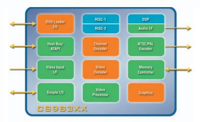
The CS983XX is a family of highly integrated DVD processors that provide all the audio and video processing functions needed for the next generation of feature-rich DVD players, DVD receivers, and Internet-based DVD applications. These processors support the playback of multiple formats, including DivX, DVD Audio, MP3, WMA, MPEG-1, MPEG-2, MPEG-4, AAC, Kodak Picture CD, Dolby® Digital ProLogic® II, Dolby® Digital ProLogic® IIx, DTS-ES,™ Dolby® Digital-EX,™ and DTS Digital Surround® decoding.
