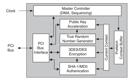
The BCM5805 security processor integrates a high-performance IPSec engine (DES, 3DES, HMAC-SHA-1, HMAC-MD5), public-key processor, true random number generator, PCI interface, and context buffer memory onto a single chip. The highly integrated BCM5805 security processor is an ideal solution for VPN-enabled networking products such as SOHO routers and gateways, VPN appliances, access concentrators, and network interface cards.
