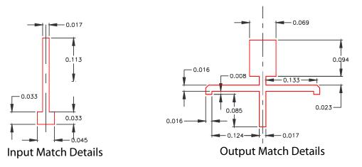
For improved performance at 6 GHz the thick transmission line (W=0.069") on the output can be extended to touch the two open stubs.
