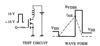
$$\begin{aligned} R_G &= 25~\Omega \\ V_{DD} &= 25~V,\, L = 398~\mu H \end{aligned} \qquad EAS &= \frac{1}{2} \cdot L \cdot I^2 \cdot \left( \frac{BVDSS}{BVDSS - VDD} \right) \end{aligned}$$
