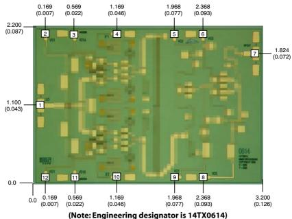
Units: millimeters (inches) Bond pad dimensions are shown to center of bond pad. Thickness: 0.110 +/- 0.010 (0.0043 +/- 0.0004), Backside is ground, Bond Pad/Backside Metallization: Gold All DC/IF Bond Pads are 0.100 x 0.100 (0.004 x 0.004). All RF Bond Pads are 0.100 x 0.200 (0.004 x 0.008). Bond pad centers are approximately 0.109 (0.004) from the edge of the chip. Dicing tolerance: +/- 0.005 (+/- 0.0002). Approximate weight: 4.36 mg.
