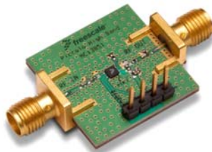
Figure 12. Typical Assembled Evaluation Board with SMA Connectors
