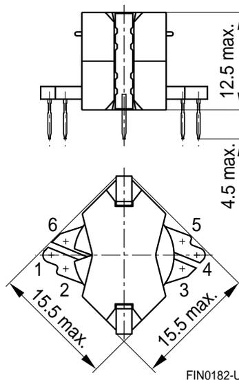
**Recommended hole arrangement (view in mounting direction)**
