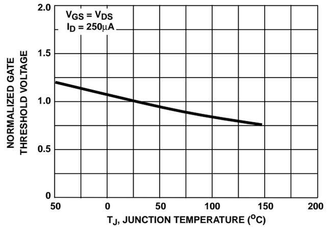
FIGURE 8. NORMALIZED GATE THRESHOLD VOLTAGE vs JUNCTION TEMPERATURE
