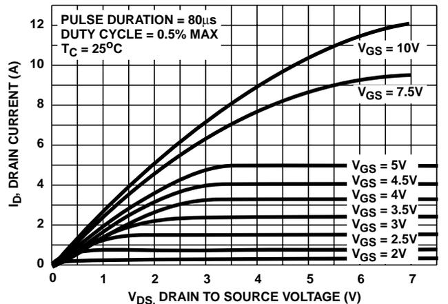
FIGURE 4. SATURATION CHARACTERISTICS
