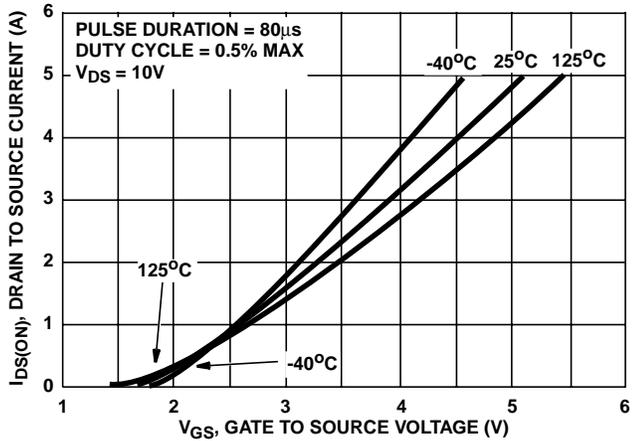
FIGURE 5. TRANSFER CHARACTERISTICS
