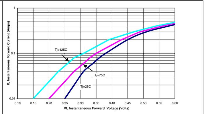
**Figure 2: Typical Forward Voltage**
