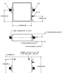
$\begin{array}{c} \mbox{Dimensions in [] are in mm.} \\ \mbox{Unless Otherwise Noted:} & .xxx\pm 0.010 [.xx=\pm 0.25] \\ .xx=\pm 0.02 [.x=\pm 0.5] \\ \mbox{WEIGHT (APPROX.): 3.2 OUNCES 90 GRAMS} \end{array}$
