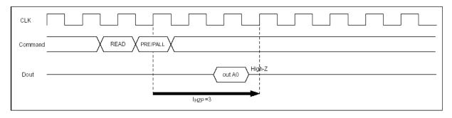
**d to Precharge command interval (same bank):** When the precharge command is executed for the same bank as the write command that preceded it, the minimum interval between the two commands is 1 clock. However, if the burst write operation is unfinished, the data must be masked by means of DQM for assurance of the clock defined by t<sub>DPL</sub>.
