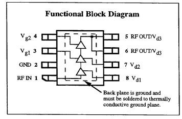
The CMM1335 is a 6 V linear power amplifier intended for use in PCS handsets, wireless local loop subscriber units and PCS base stations. As a pin-compatible member of the new *Triniti DX™* amplifier family, the CMM1335 offers maximum performance and flexibility. The flexible amplifier can be biased to support the requirements of PCS-1900, IS-136, IS-95 or DCS-1800 systems.
