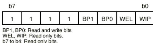
The BP1 and BP0 bits in the status register can be used to write protect a block of memory. In this application, both bits are cleared, allowing write access to all the memory.
