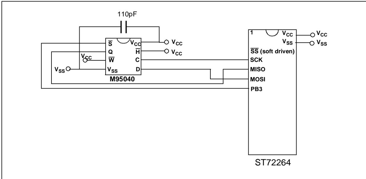
$\overline{SS}$  pin of ST72264 is software driven (high state for a master device).
