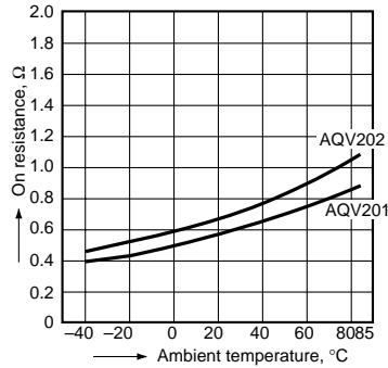
2.-(4) On resistance vs. ambient temperature characteristics
