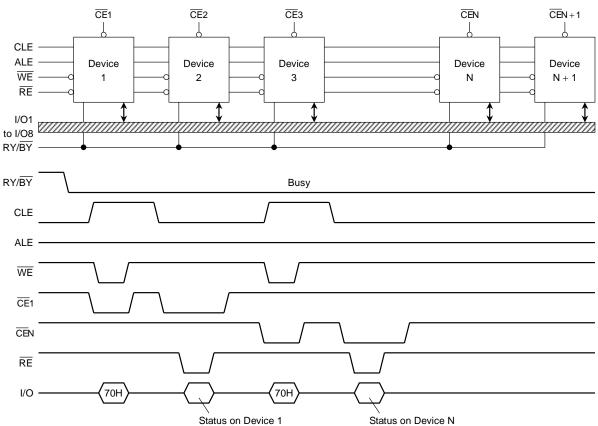
Figure 6. Status Read timing application example
