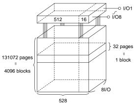
Figure 2. Schematic Cell Layout
