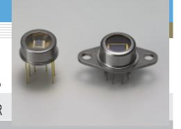
S2592/S3477 series sensors combine a UV to near infrared Si photodiode with a thermoelectric cooler. A thermistor is also included in the same package to sense the Si photodiode chip temperature. This allows stable operation over long periods of time, making these sensors suitable for low-light-level detection where a high S/N is required.
