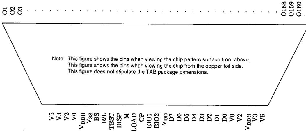
Note: In the LC4104TAB-02 version of this product, the TEST pin must be left open (no connections).
