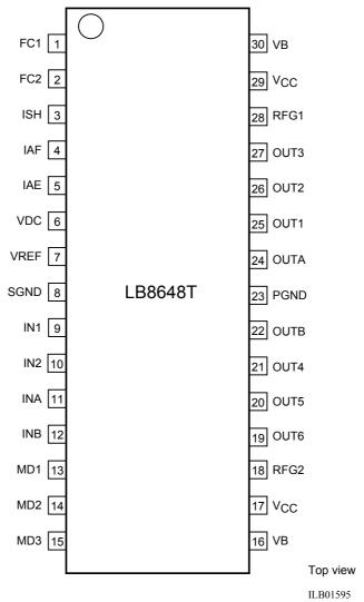
Note) V<sub>CC</sub> and VB, both 2 pins are connected.
