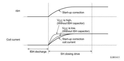
The ISH pin input voltage is set with the decay time constant by using the external CR. By setting the voltage to be lower than the coil decay time constant, the start-up wave of coil current is determined from the decay time constant of the external CR. By doing this, stable shutter operation can be carried out with respect to the power supply variations.
