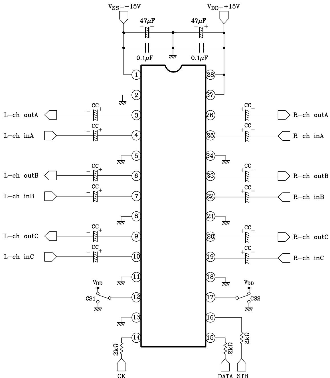
(\*) CC indicates the capacitor from  $1\mu F$  to  $10\mu F$ .
