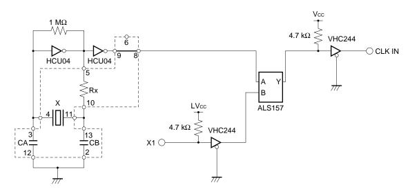
Remark The sections enclosed in broken lines indicate parts that are attached to the parts board.
