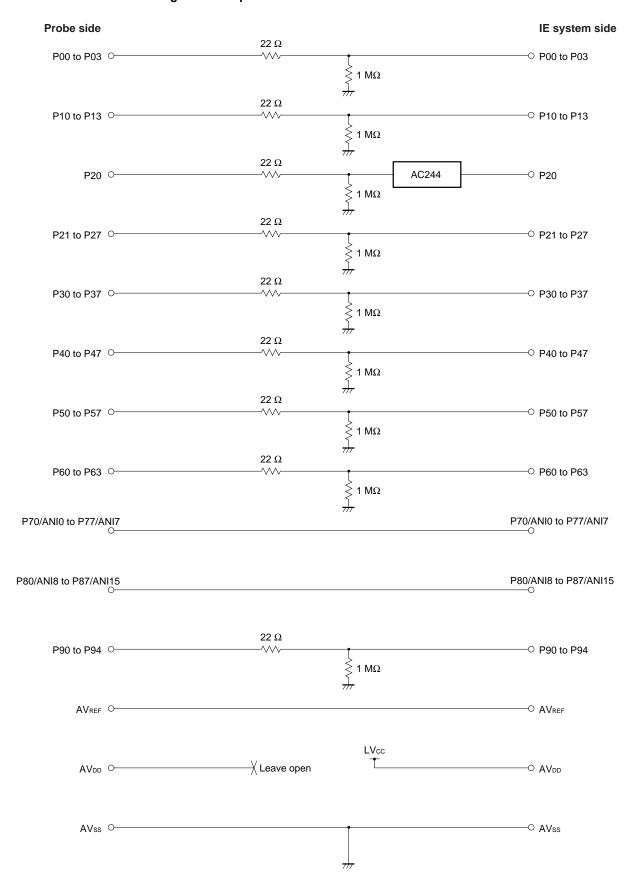
Figure 4-1. Equivalent Circuit 1 of Emulation Circuit
