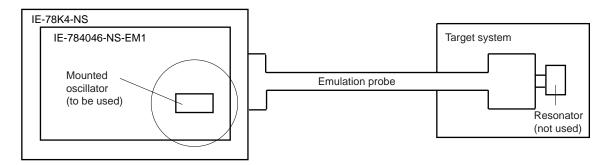
Remark The clock that is supplied by the IE-784046-NS-EM1's oscillator (encircled in the figure) is used.
