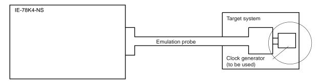
Remark The clock supplied by the target system's clock generator (encircled in the figure) is used.
