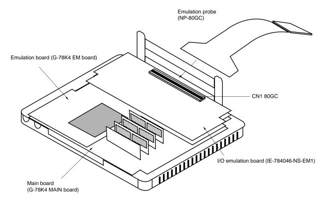
Figure 3-1. Connection of Emulation Probe
