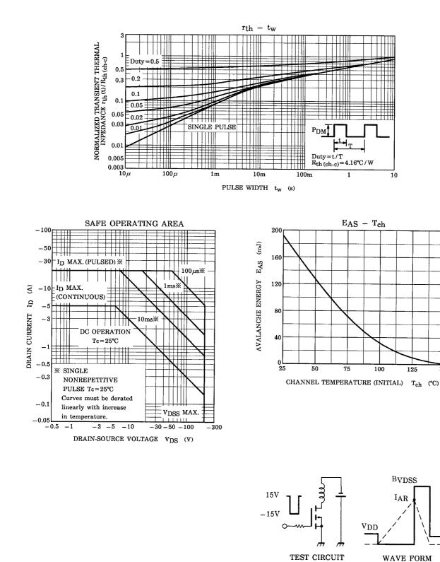
$E_{AS} = \frac{1}{2} \cdot L \cdot I^{2} \cdot (\frac{B_{VDSS}}{B_{VDSS} - V_{DD}})$
