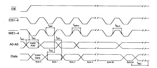
Note: (1) A6 through A14 must specify the page address during each high to low transition of WE1~4 (or CS1~4).
