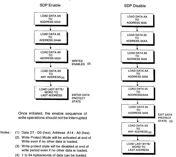
Note: Load Data above represents 8 bit mode. For 16 or 32 bit mode, place the load data in the 2 bytes or all 4 bytes on the data lines, respectively. Eg/ 8 bit load data =  $55_{HEX}$ , 16 bit load data =  $5555_{HEX}$ .
