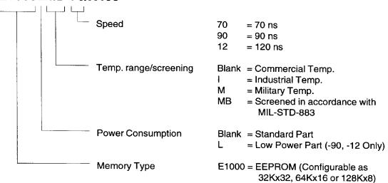
NOTES: 1. X405 indicates customer specific part. X405 is designed for Fast Page Write applications.  $t_{wc}$  = 3ms (Max.). If not specified when ordered only a  $t_{wc}$  of 10ms (Max.) can be guaranteed.
