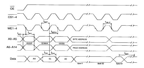
Notes: (1) A6 through A14 must specify the page address during each high to low transition of WE1~4 (or CS1~4). (2) OE must be high only when WE1~4 and CS1~4 are both low.
