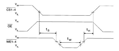
$$t_{_{S}} = t_{_{H}} = 5 \mu s \text{ (min)} \quad t_{_{W}} = 10 \text{ ms (min)} \quad V_{_{H}} = 12 V \pm 0.5 V$$
